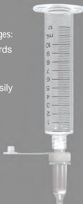
Syringe as reservoir connected to Luer-lock cap of Mobicol
